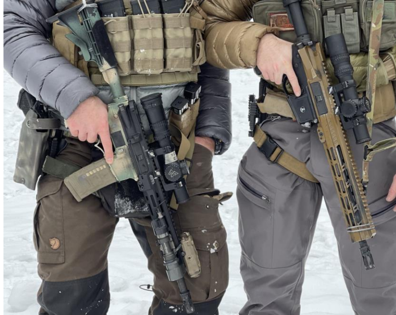
Figure 43: 12.5" Mid Gas System in 5.56mm (L) and 12.5" Piston System in 5.56mm (R)
