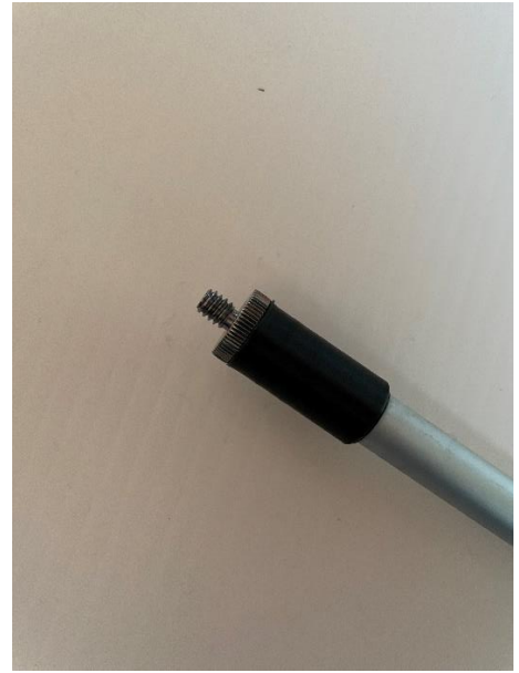
Spike with 6mm thumb screw to stop rotation. Top attachment with 1/4 inch screw.
