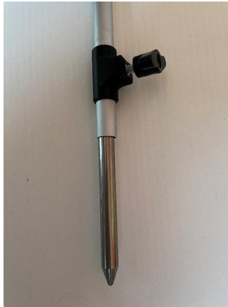
Spike with 6mm thumb screw to stop rotation. Top attachment with 1/4 inch screw.
