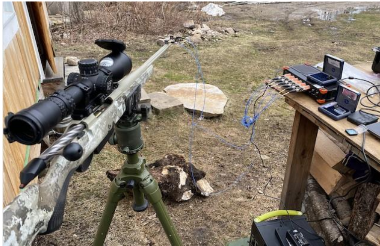
Figure 30: Tikka System Rifle Barrel Test, DEWESoft DAQ, PCB Accels
