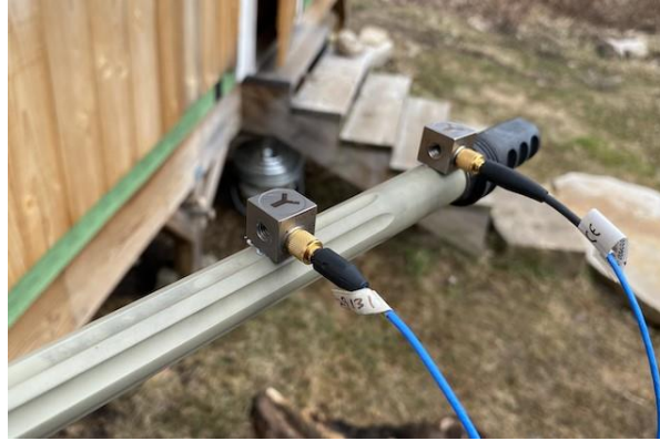
Figure 33: Tikka System Rifle Barrel Test, Accelerometer Placement
