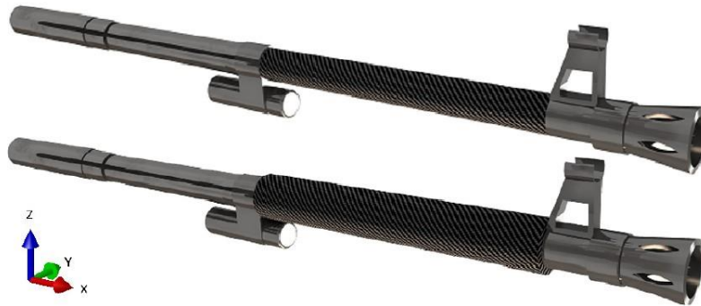
Figure 6: Carbon Fiber Wrapped Machine Gun Barrels, Pyka et al., 2019
